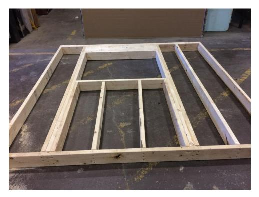
Construction of the specimen (Specimen #2)
